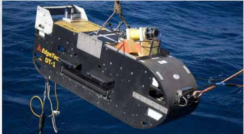
EdgeTech's 2400 Series is a fully integrated combined side scan sonar (with optional wide swath bathymetry) & sub-bottom profiling system designed for deep water operation in depths down to 6,000 meters.
